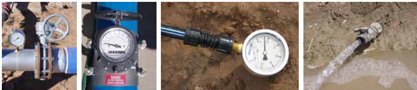
From left to right: Pressure gauge on mainline; flow meter; pressure gauge on tape; monitoring tape flush water.
